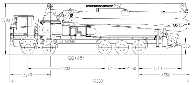
Note: Serial version. Dimensions and weights depend on truck pump model and equipment. Dimensions in mm, MB-Actros 5050 as example
